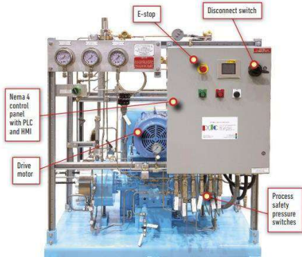
PDC-3-300-7500 two-stage compressor, helium gas, Industrial Gas Industry, 517 barg/7,500 psig discharge pressure, 20 Nm 3 /hr flow rate, 7.5 kW/10 HP motor.
